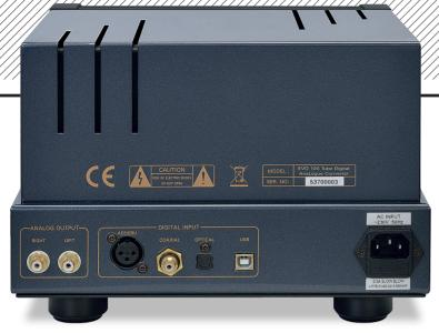
ABOVE: Simplicity itself – four standard digital inputs are fitted including AES/ EBU (XLR), S/PDIF (on RCA and optical) and USB-B for computer connection. Fixed, transformer-coupled analogue outputs are on single-ended (RCA) connections only
